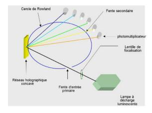
This technique involves erosion during the analysis, so it is adapted for distribution depth profiling (evolution of the intensity of the characteristic lines of the followed elements, as a function of erosion time). As the erosion speed depends on the element and on the matrix, Science et Surface develops multi-elements and multi-materials calibration methods so that most of profiles will be quantitative.
